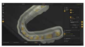
Support structures as well as drainage canals and vents are automatically placed by the software but can also be added, removed, and repositioned manually.
