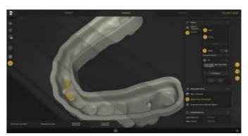
The software indicates where air may potentially get trapped during the wash process later on or where puddling of resin may occur, which might not be cleaned up. In this case, drainage canals can be positioned virtually, based on the planned print placement, directly in the CAM software without the need to go back to the design phase.
