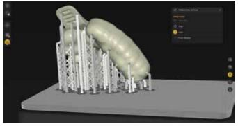
Depending on the application and its desired surface quality, different thicknesses can be defined with the appropriate detail level, thereby optimizing print times.
