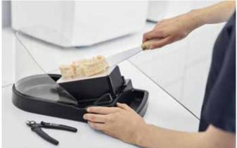
The completed printed objects are attached to the building platform with the support structures and can be removed quickly and easily with just a few moves. The Primeprint Solution Platform Holder is specially designed to make removal even easier. It anchors the building platform in a non-slip manner and catches detached print parts.
