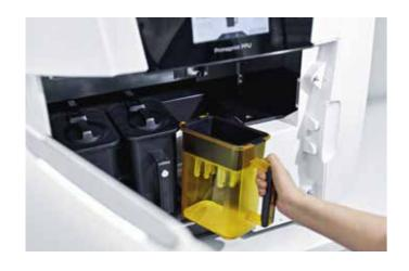
After the print is completed, only the Primeprint Box is removed from the printer and placed into the PPU. The Primeprint Box is sealed and protected from UV light; it does not require any additional contact precautions. Based on the RFID identifier, the individual job is detected and the fully automated post-processing begins with just one click on the screen. The rest is taken care of by the PPU.
