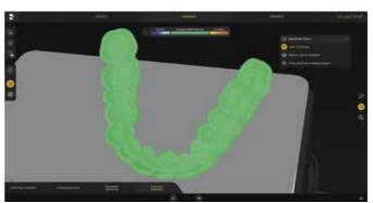
For quality enhancement, the software indicates compliance or noncompliance with manufacturer-specified wall strength – a special advantage of the validation process that was performed for each Primeprint material. As such, additional corrections can be made, for example in the case file when cases of noncompliance are detected.
