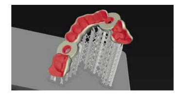
In addition to purely geometrical generated design data, CEREC and inLab CAD Software contains additional specific dental information regarding application aspects, such as functional areas and important geometries, which require special consideration during the 3D printing process. For 3D prints with Primeprint Solution, the CAM software algorithm detects and applies this specific dental information to optimize the print job.
