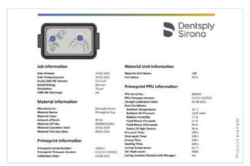
A quality process protocol documents the manufacturing process for each medical device produced with Primeprint Solution. In addition to the simplified distributor declaration of MDR conformity, it can be used as proof of compliance with the process specifications validated by the material manufacturer.
