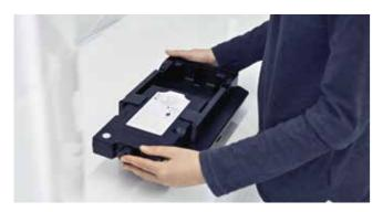
The Primeprint Material Unit consists of the vat and the insertion slot for the material cartridge. The material cartridge clicks into the material unit with a hand movement. Both the vat and the material cartridge are fitted with RFID tags. Once assembled, the software automatically pairs them and identifies them as a unit.
